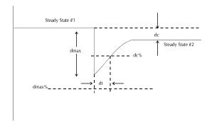
A steady state voltage that undergoes a voltage change (dmax), exceeding the limit dc% for a time dt seconds (but staying within the limit dmax%), before returning to a second steady state dc voltage level (which is less than dc%, with dt being less than 200ms), will pass the dc, dmax, and dt voltage deviations test.
