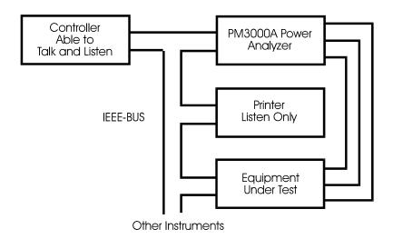
The IEEE-488 bus consists of a controller (e.g. a computer with an IEEE card) and one or more instruments. These may be talkers (able to send results), listeners (able to receive commands) or talker-listeners (able to receive commands and send results).
